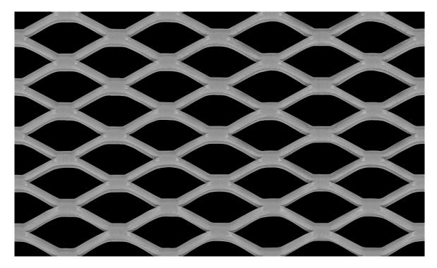
LW Aperture:27.00mmStrand Width:3.25mmSW Aperture:12.20mmThickness:3.00mmWeight:8.06 kg / m2Open Area:65%
